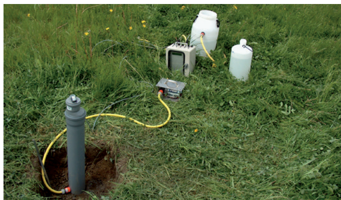
Essai open-end (CRR, 2008)
