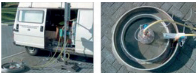
Essai au double anneau (CRR, 2008)
