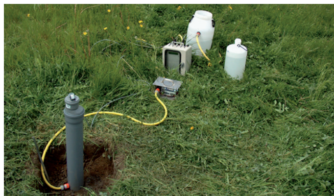
Essai open-end (CRR, 2008)
