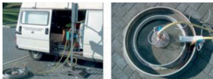
Essai au double anneau (CRR, 2008)
